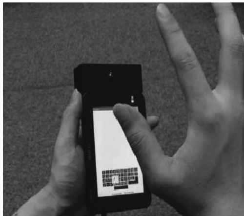
Figure 2.17 – In-air typing interface of Fastfinger [60].
