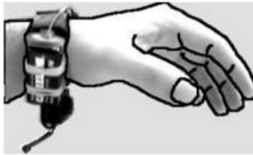
Figure 2.18 – UbiHand wrist-worn input device [2].
