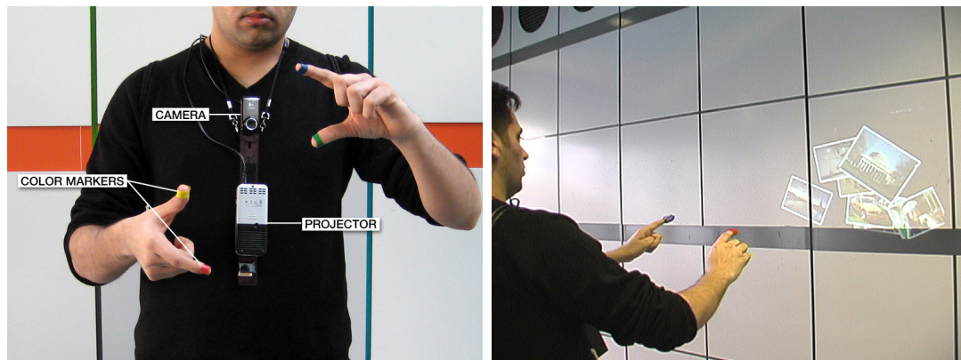
Figure 2.21 – The Sixthsense system uses a camera and a projector to convert any surface in an interactive surface [42].
