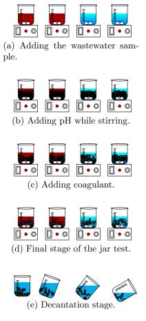
Figure 2.2: The principal steps of the jar test.
