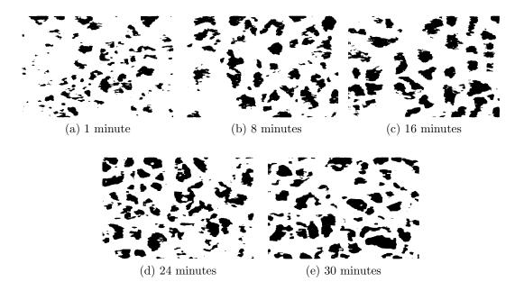
Figure 4.2: Microscopic images of the flocculation process, for the data set 2, observed at five different agitation times for iron chloride at an agitation speed of 25 rpm.
