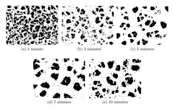
Figure 4.1: Microscopic images of the flocculation process, for the data set 1, observed at five different agitation times for iron chloride at an agitation speed of 20 rpm.
